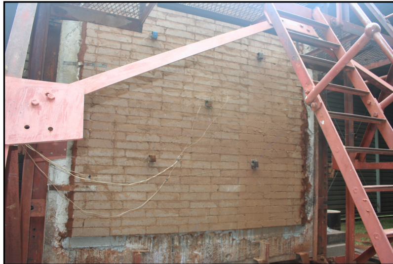
Figure 3.1: Wall test specimen as seen from unexposed side prior to test
