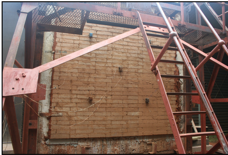
Figure 3.3: Unexposed side of test wall upon termination of the test
