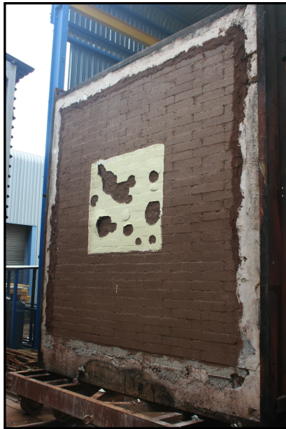
Figure 3.4: Exposed side of test specimen immediately after removal from furnace
